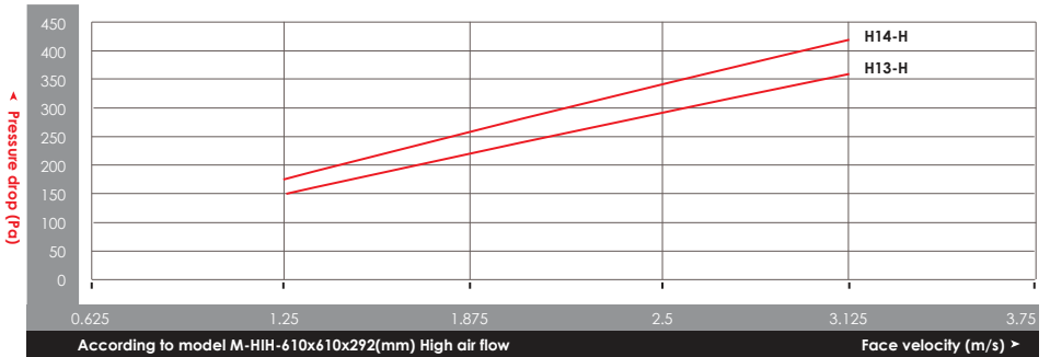
Graph Of Initial Pressure Drop Versus Face Velocity (High Air Flow & Low Pressure Drop)
